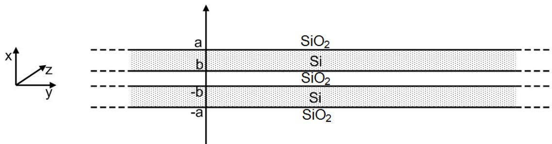
Figure 2: Slot waveguide made of silicon and silica.
